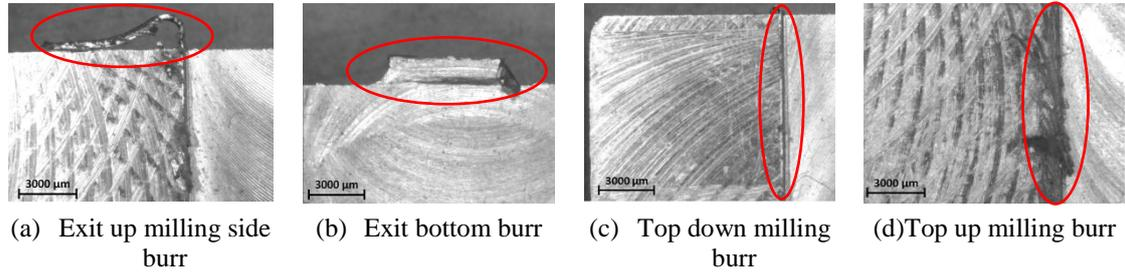
Figure 2; Investigated slot milling burrs
