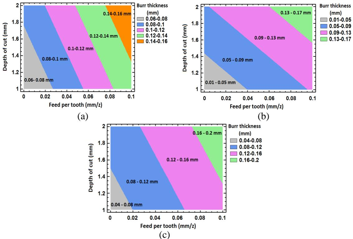
Figure 4; 2D contour plot of  $B_{t,1}$  as function of feed per tooth and depth of cut at fixed cutting speed 1200 (m/min) when using : (a) Tool 1, (b) Tool 2, (c) Tool 3
