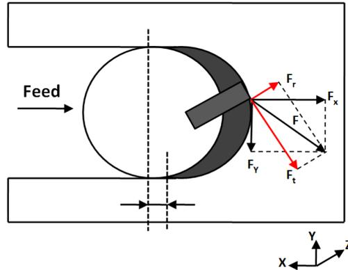
Figure 5; Slot milling under orthogonal cutting conditions
