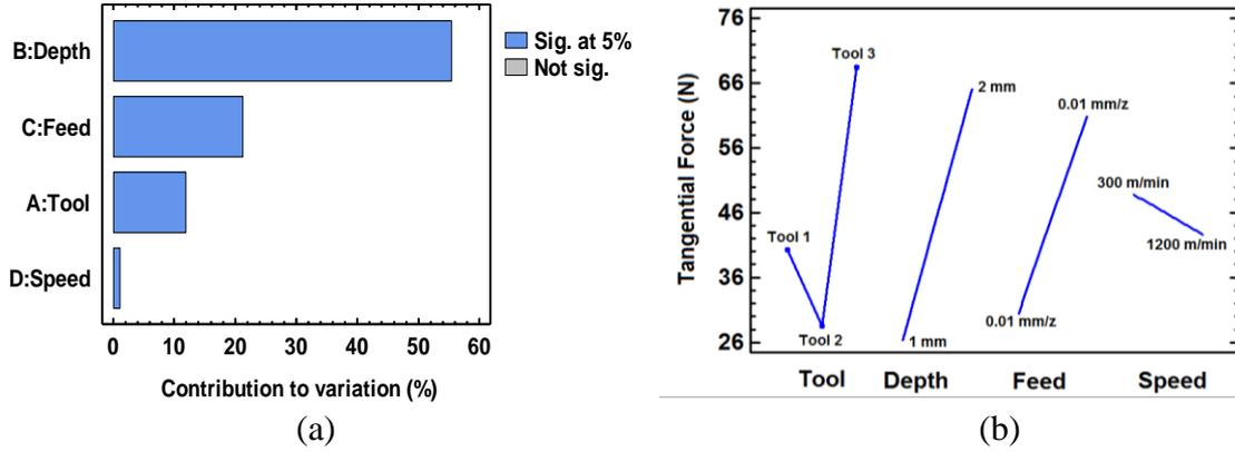
Figure 6; (a) Pareto chart  $F_t$  in linear design model, (b) Direct effect plot for  $F_t$
