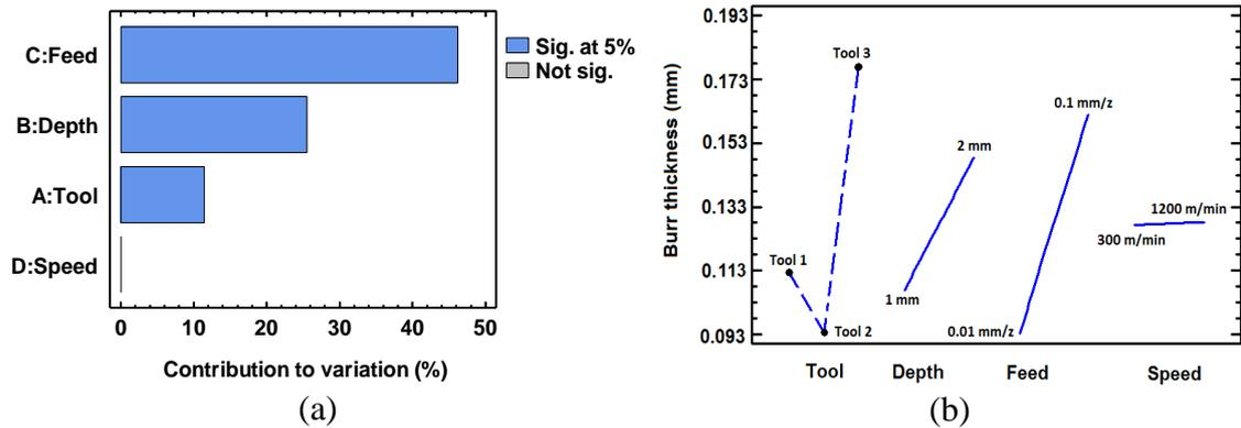
Figure 3;(a) Pareto chart for  $B_{t,1}$  in linear design model, (b) Direct effect plot for  $B_{t,1}$
