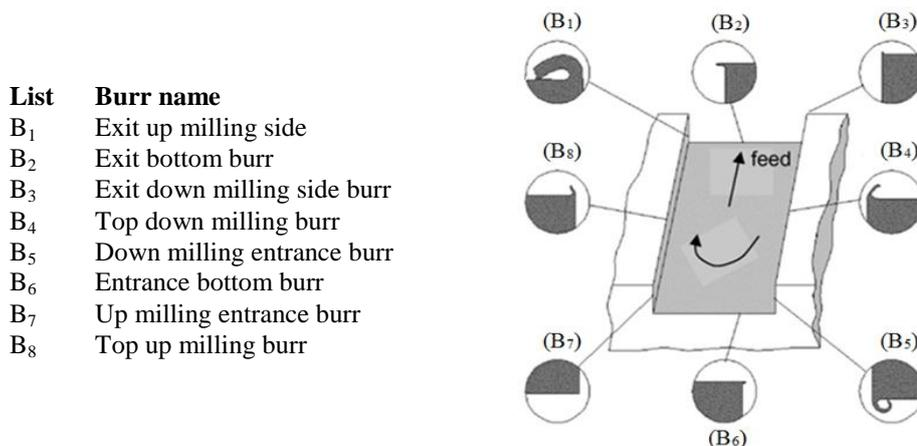
Figure 1; slot milling burrs
