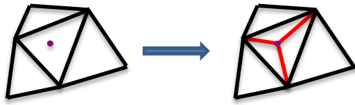
Figure 3: Violet point is inserted into a mesh by incremental Delaunay triangulation method.
