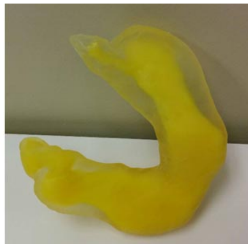
Material jetting method and resulting stomach fabrication
