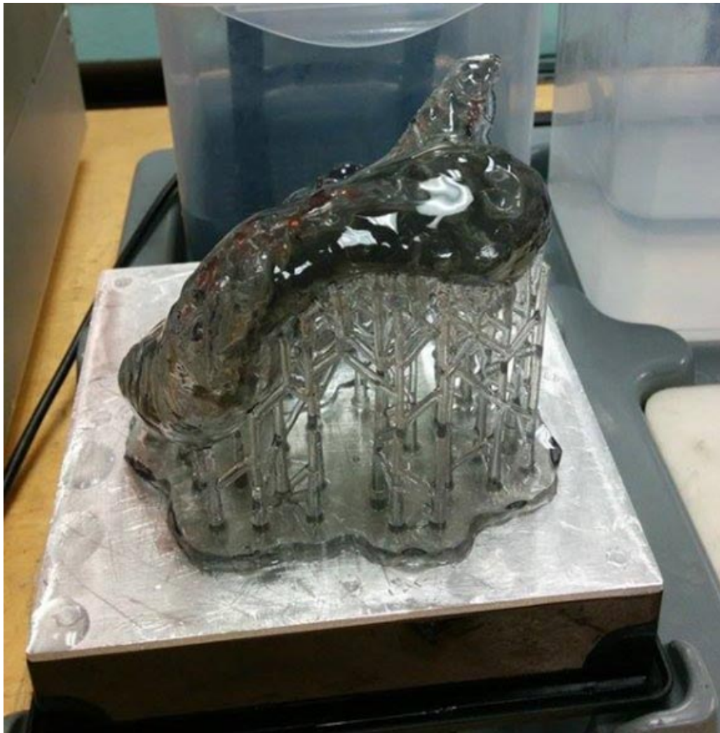
Stomach made by photopolymerization
