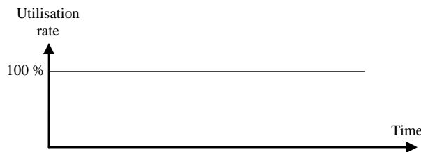
Figure 2: Work load of a production machine when transfer time is negligible
