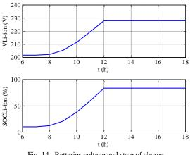
Fig. 14 Batteries voltage and state of charge
