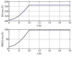
Fig. 16 Batteries voltage and state of charge
