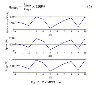
With the MPPT algorithm used in this work, an efficiency of 98.63% is achieved despite the sudden change of illumination (from 800W/m<sup>2</sup> to 100W/m<sup>2</sup>during one hour).
