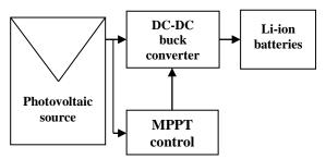
Fig.2 Block diagram of the photovoltaic system
