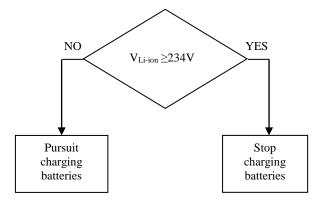
Fig.11 Principleof the supervision system
