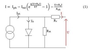
Fig. 4 Equivalent circuit of a photovoltaic cell
