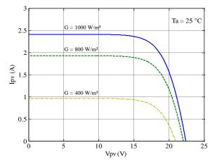
Fig.6 Effect of illumination on the characteristic current-voltage
