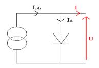
Fig. 5 Simplified equivalent circuit of a photovoltaic cell Properties of the selected PV panel are given inTable II.
