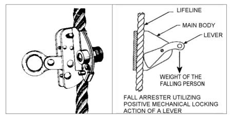
Figure 2: Fall arrester and its cam lever mechanism
