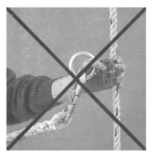
Figure 3: Grasping the lever of the fall arrester
