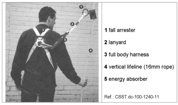
Figure 1: Individual fall arrest system
