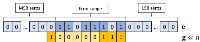
FIGURE 5. Illustration of the error range applied to CRC-CCITT-8 ( n = 8 ). Canceling LSB non-zero values by performing an XOR operation with a generator polynomial of width n + 1 bits produces an error range of n bits.
