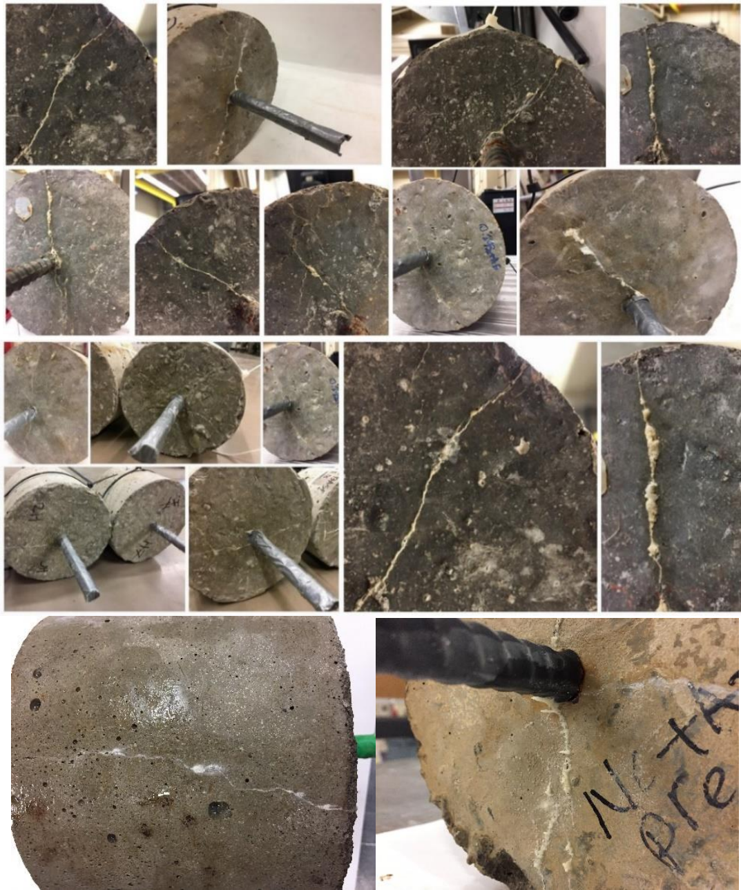
Fig. 19 Healing products at the external crack surface of pull-out specimens of SAP-based NC mixtures with and without AE
