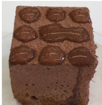
Figure 6-7 Water repellence of an earth mortar stabilized by microbially induced iron-oxide precipitation (MIIP) (Faria and Lima, 2018)
