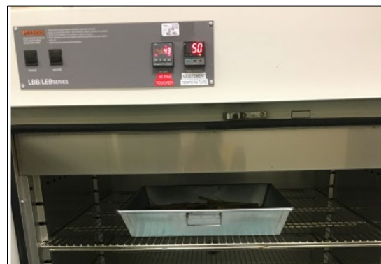
Figure 5: Drying the fibres at 50 °C.
