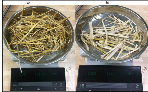
Figure 4: Samples of wheat fibre (a) and corn stalk fibre (b) before placing in the oven.
