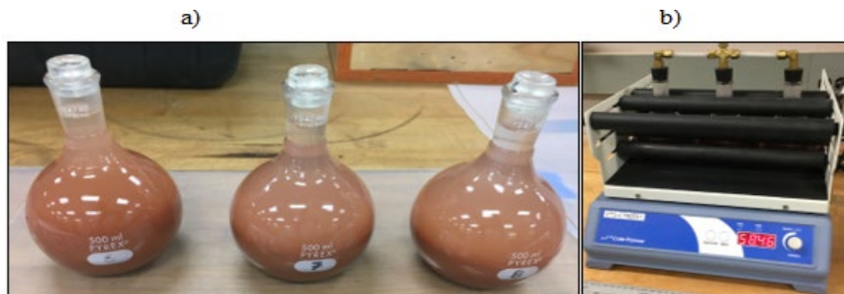
Figure 3: Samples of red clay for tests (a) and removal air bubbles (b)
