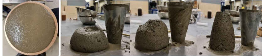
Fig. 1. Top view of the flow table (a), side view of the slump test (b, c, d).
