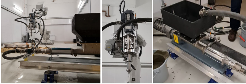
Fig. 3. The large-scale additive manufacturing laboratory of ETS and the extrusion system used in this study (a), the extrusion head (b), and the progressive cavity pump (c).
