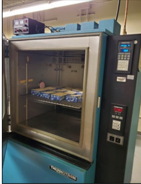
Fig. 2. Moisture Buffering Value Test in Thermotron environmental chamber.
