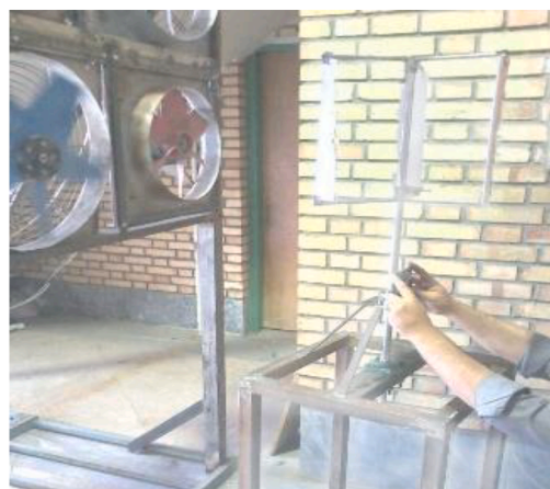
Fig. 9. Experimental setup: (a) schematic and (b) the test turbine.
