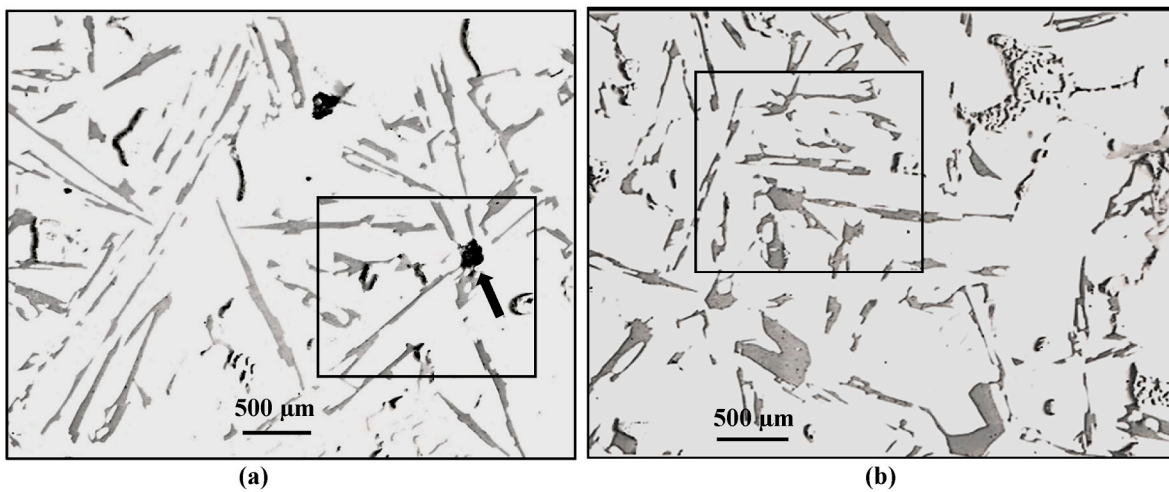
Fig. 10. Morphology of eutic Si plaquettes in samples poured from:(a) 750 °C, (b) 950 °C.
