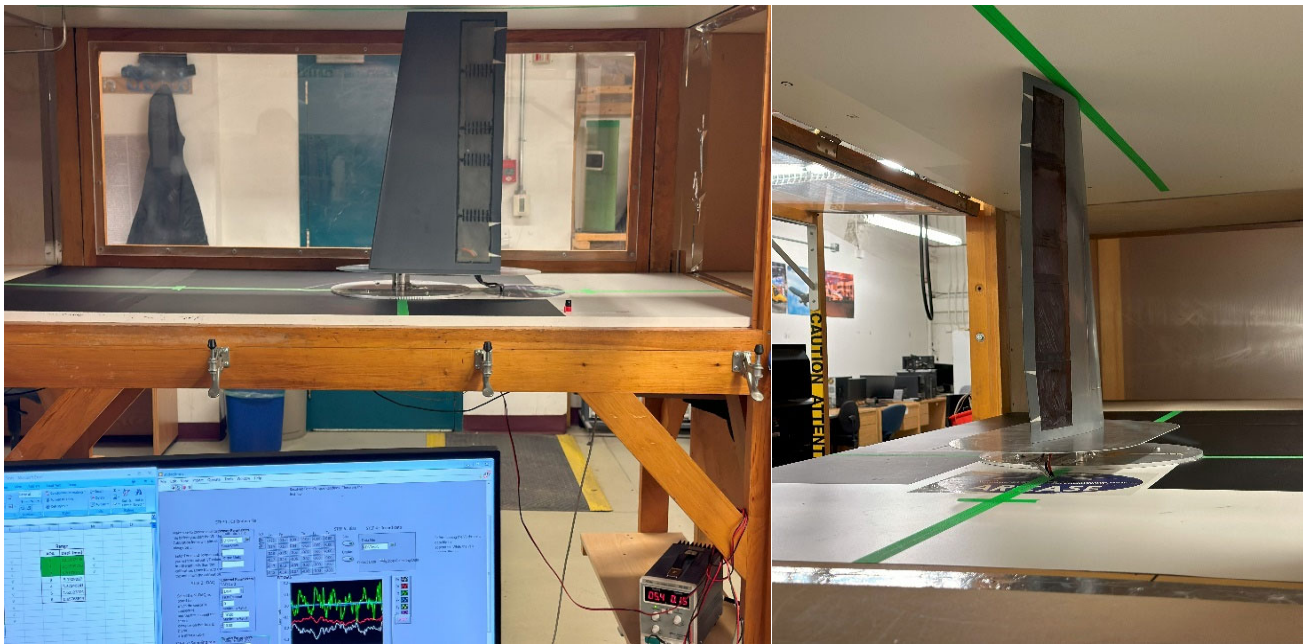
Figure 20. UAS-S45 morphing wing section installed in the wind tunnel test section.
