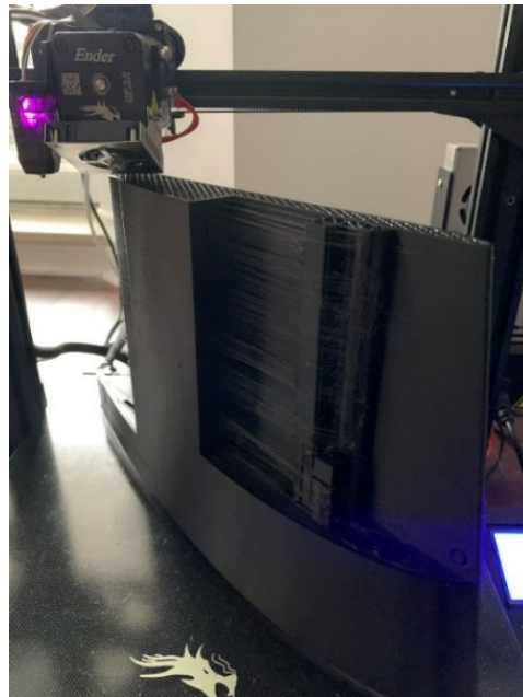
Figure 5. Three-dimensional printing of the wing section with vertical arrangement.
