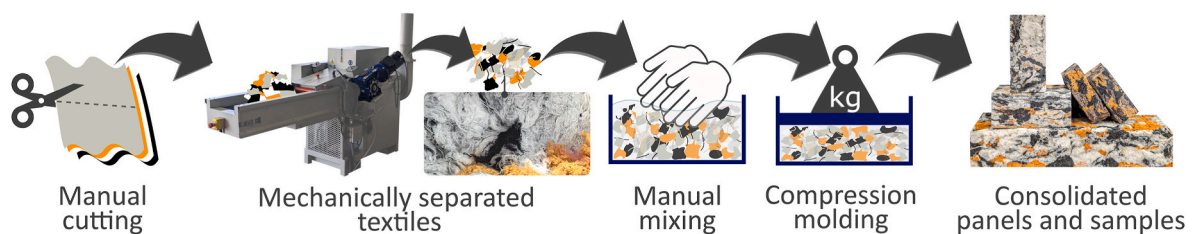
Fig. 2. Schematic illustration of the fabrication process from fabric to textile composite panels.
