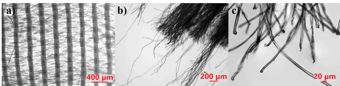
Fig. 3. Morphology of a) fabric, b) yarn, and c) fibers after mechanical transformation using OM.
