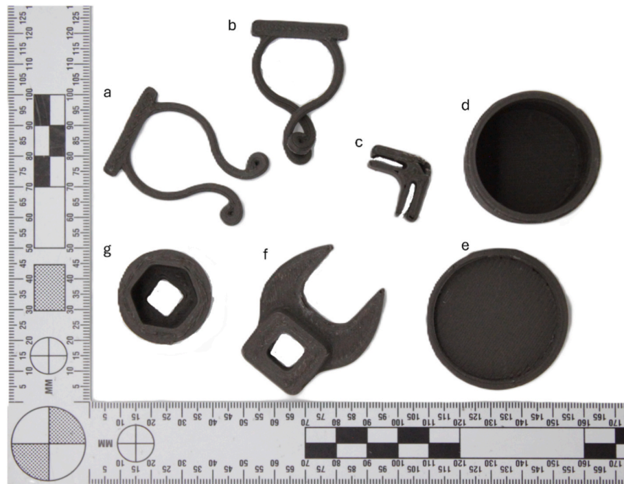
Fig. 9. Photograph of 3D printed tools designed by NASA: a-b) wire tie; c) cube sat clip; d-e) container and lid with interlocking thread; f) crowfoot; and g) torque tool. All the parts are printed with composite containing 30 wt% regolith.
