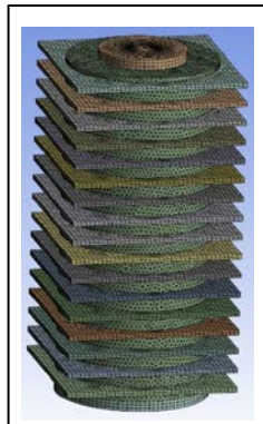
Figure 2: The mesh distribution of the battery cell with the maximum number of fins.
