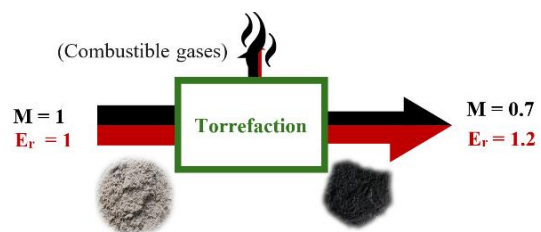
Figure 1. Schematic Principle of Torrefaction
