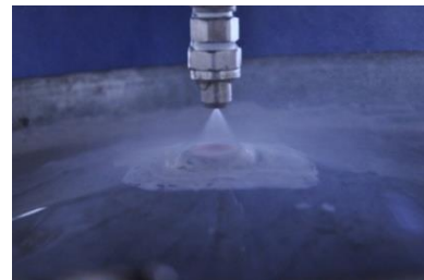
Figure 2 Direct photograph showing the impingement zone during spray impingement.
