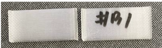
Figure 2. 3D printed PETG sample breaking at interlayer bonds, as expected.
