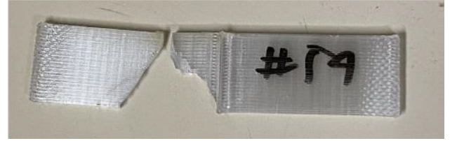
Figure 3. 3D printed PETG sample not breaking at interlayer bonds.
