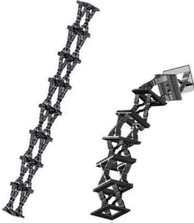
Figure 6. Original and deformed robot arm
