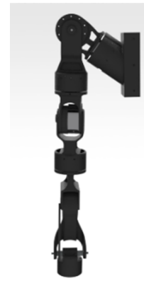
Figure 1. The GRASP-01 humanoid robotic arm has optimized geometrics designs, achieving a total system mass of 5.6 kg. The modular architecture enables future geometric refinements for enhanced performance characteristics
