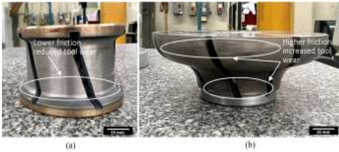
Figure 8. Comparison of the tool wear : (a) Eased concave shape reduced tool wear, (b) Ogee edge shape increased tool wear
