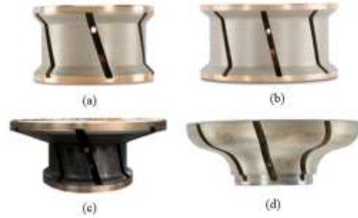
Figure 2. Experimental used abrasive tools: (a) Eased chamfered edge tool, (b) Half-beveled edge tool, (c) Eased concave edge tool, (d) Ogee edge tool
