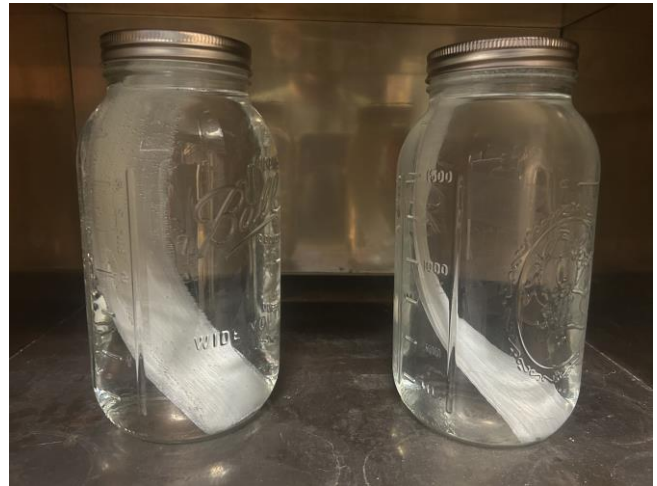
Figure 1: Samples inside glass jars for aging at 95°C in DW and DI water.
