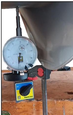
Figure 5. Dial indicator mounted to apparatus and engaged on the Archimedes screw's inner cylinder.
