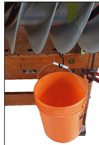
Figure 6. A 20 litre bucket was filled with water to increase and decrease loading for the validation experiments.
