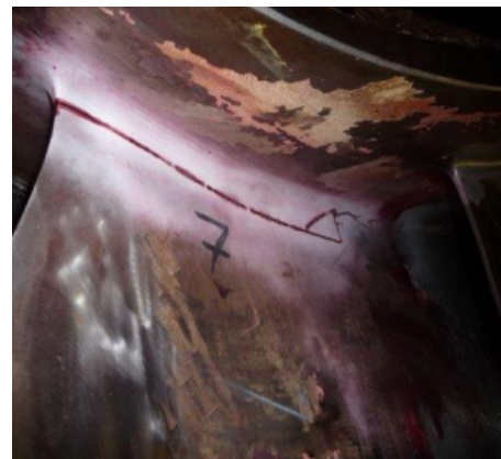
Figure. 1. Cracks on Francis runner blade.
