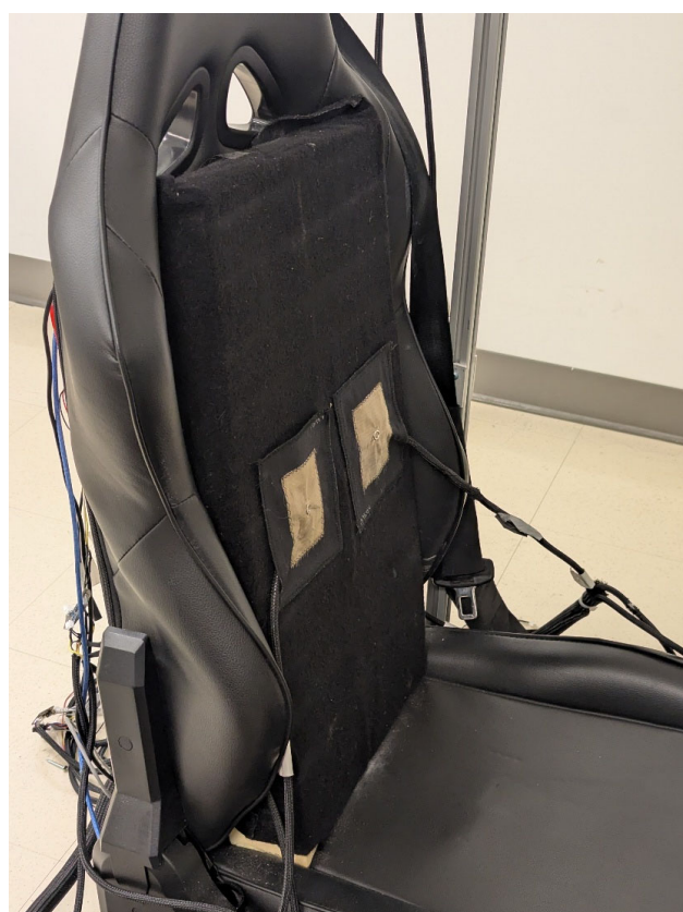
Figure 8. Picture of cECG textile electrodes fastened on the seat back.
