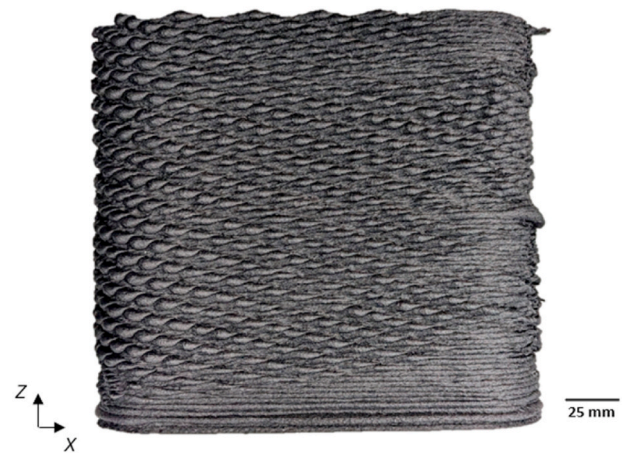
Fig. 16. FGF box printed using parameters of Table 2 with the twice-recycled pellets (pellets obtained from shredded printed boxes).
