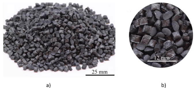
Fig. 2. CF/PEKK-PEEK recycled pellets made from CF/PEKK pre-impregnated tape edge trims.
