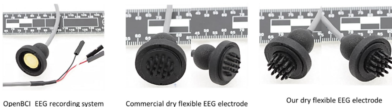
FIGURE 3 | Electrodes installed in the system for the acquisition of electrical signals from the brain. [Color figure can be viewed at wileyonlinelibrary.com ]
