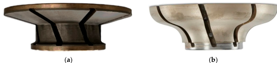
Figure 2. Experimental used abrasive tools: (a) Half-Beveled tool; (b) Ogee tool.
