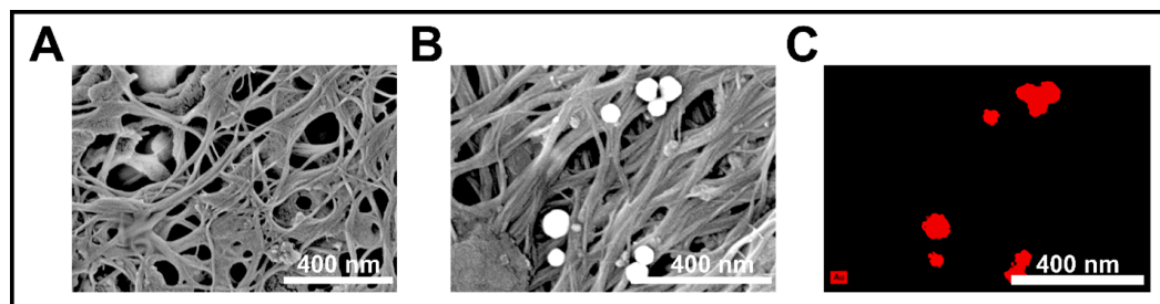
Figure 5. (A) SEM image of the bare CNT membrane showing a porous fibrous structure with nanoscale interconnections. (B) SEM image after AuNP exposure, revealing uniformly distributed spherical gold nanoparticles embedded on the CNT network. (C) EDS elemental mapping confirming the presence and distribution of Au (shown in red) on the CNT surface, indicating successful nanoparticle trapping via surface interaction.
