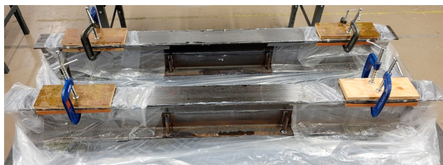
Figure 3. Curing of the SikaWrap fabric.
