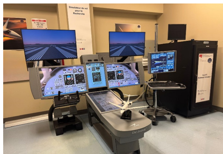
Figure 1. Research Aircraft Flight Simulator of the Cessna Citation X available at the LARCASE laboratory. The flight simulator is qualified to Level D for its flight dynamics.
