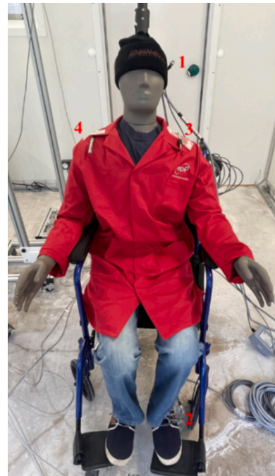
Fig. 4. Seated thermal Manikin Newton®.
