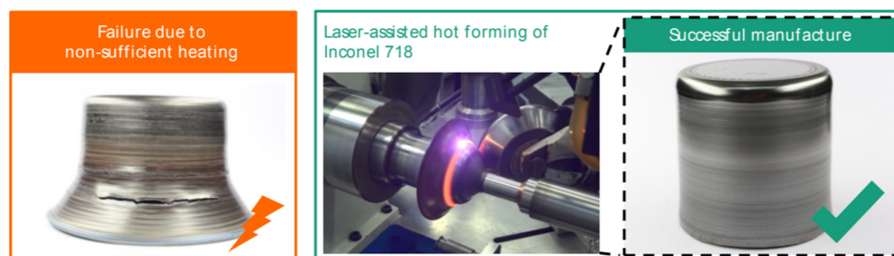
Figure 4. Comparison between cold and laser-assisted metal spinning of Inconel 718. Insufficient heating during conventional forming results in circumferential cracking and part failure (left), while laser-assisted hot forming enables successful multi-pass spinning with improved formability and surface quality (right). Reproduced from [29] under CC by 3.0.
