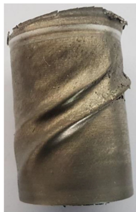
Figure 25. Overheating-induced geometric defects in hot spinning: excessive temperature and uneven deformation soften the wall and trigger warping in AZ31 flow forming. Reproduced with permission from [70].
