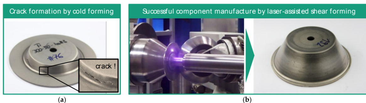
Figure 21. Impact of laser assistance on shear forming. (a) Cold spinning at room temperature leads to crack initiation due to high work hardening and limited ductility. (b) Crack-free component produced by laser-assisted shear forming. Reproduced from [29] under CC by 3.0.
