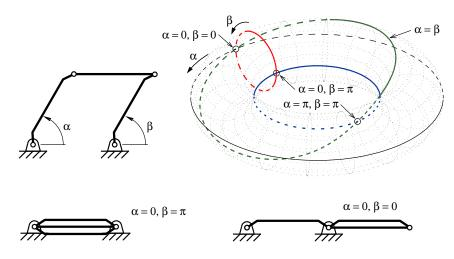
Figure 1. The equal-length four-bar mechanism, the C-space and its singularities.
