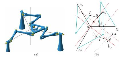
Figure 3. The planar mode: (a) face up; (b) C-singularities face down.
