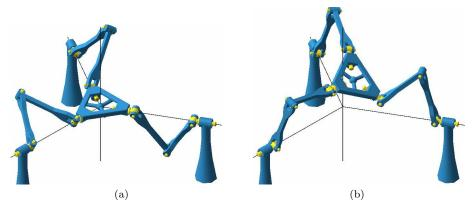
Figure 4. The DYMO chain in (a) lockup mode and (b) mixed mode.
