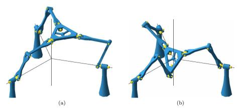
Figure 2. The DYMO chain in (a) translation mode and (b) orientation mode.
