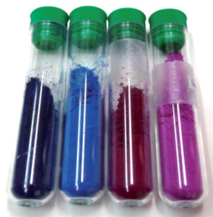
Fig. 2 Resulting sepiolite pigment: MB ss , MB as , MR ss , MR as (from left to right).
