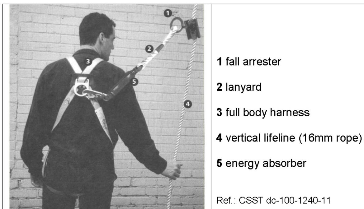
**Figure 1: Individual fall arrest system**
