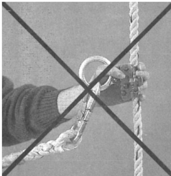
**Figure 3:** Grasping the lever of the fall arrester
