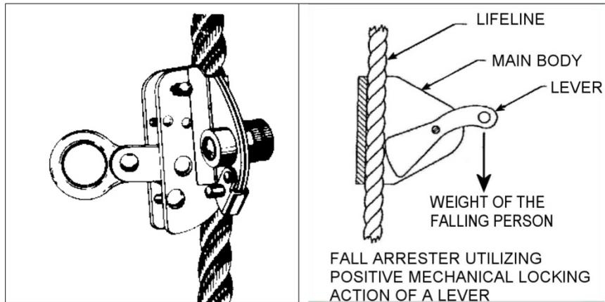
**Figure 2:** Fall arrester and its cam lever mechanism
