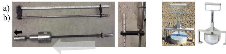
Figure 1. Measurement of the consolidation of CLSM, a) dynamic cone penetrometer, b) ball drop (Kelly ball)
