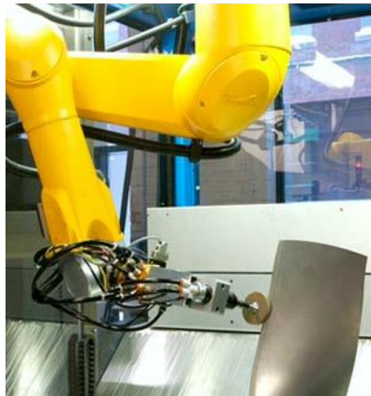
Figure 17. A robot arm combined with deburring brush [30]
