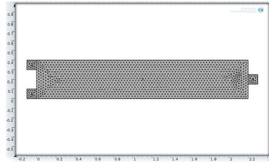
Figure 1. Meshing of the diluter in COMSOL
