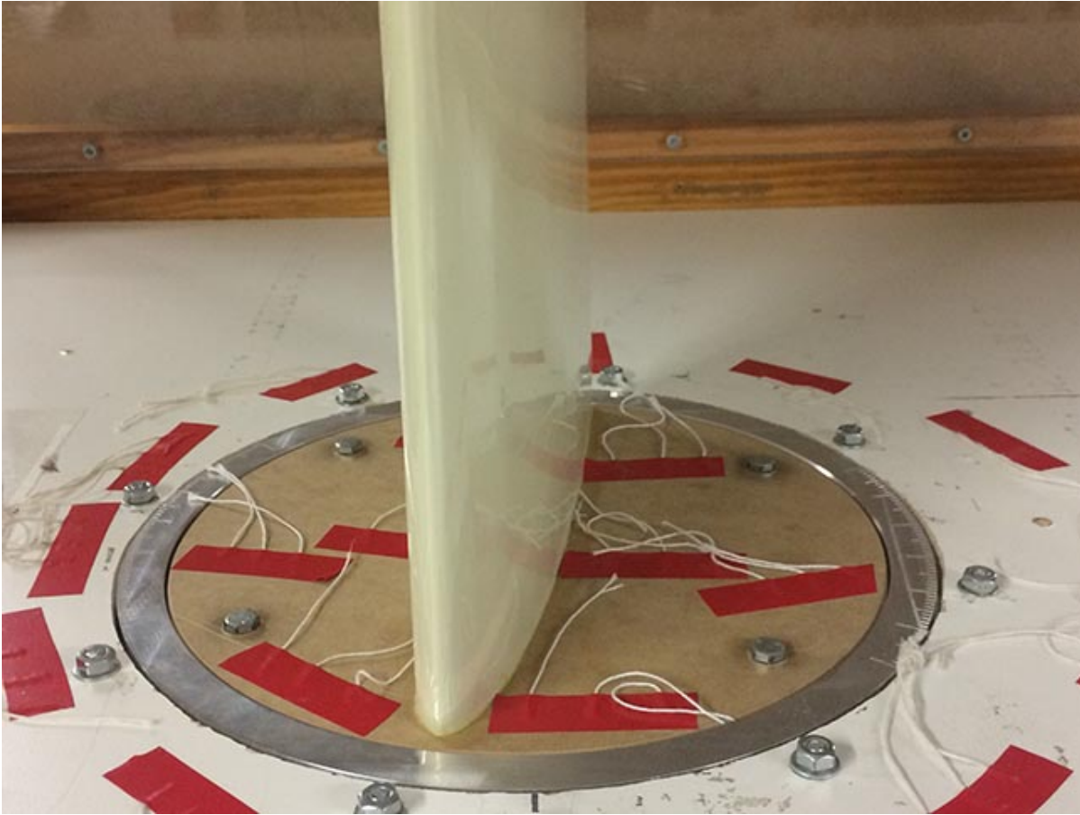
Figure 1 Part of a wing placed on the carrier plate of the balance inside the wind tunnel
