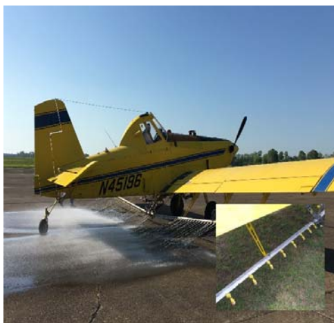
Figure 2 Air Tractor 402B with CP-11TT nozzle booms
