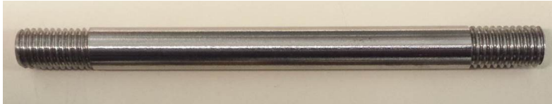
Figure 1. Solidification sample prepared from the hot top of 40 MT of high strength low alloy steel
