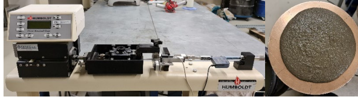
Fig. 2. The modified direct shear apparatus (a) and top view of the flow table (b).
