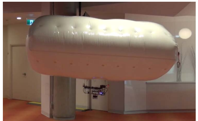
FIGURE 1: Our blimp design; a pillow-shaped polyurethane bladder with internal strings to maintain its shape and a suspended gondola with all its mechatronics underneath.
