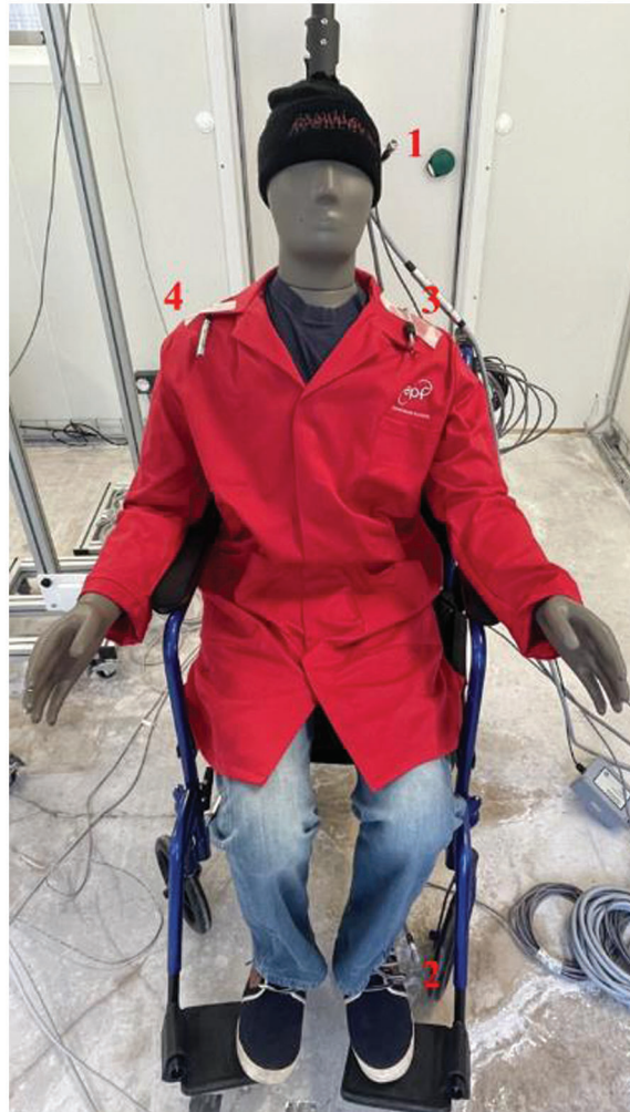
Figure 6: Location of the ambient sensors on the manikin. The Amb Temp1 sensor and Amb Temp2 sensor are placed on the head and ankle of the manikin, corresponding to 1 and 2 in the figure. The air velocity sensor and relative humidity sensor are placed on the shoulder of the manikin, corresponding to 3 and 4 in the figure, respectively
