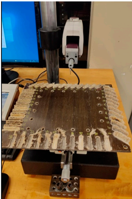
Figure 7. Mitutoyo surftest SJ-410 profilometer.
