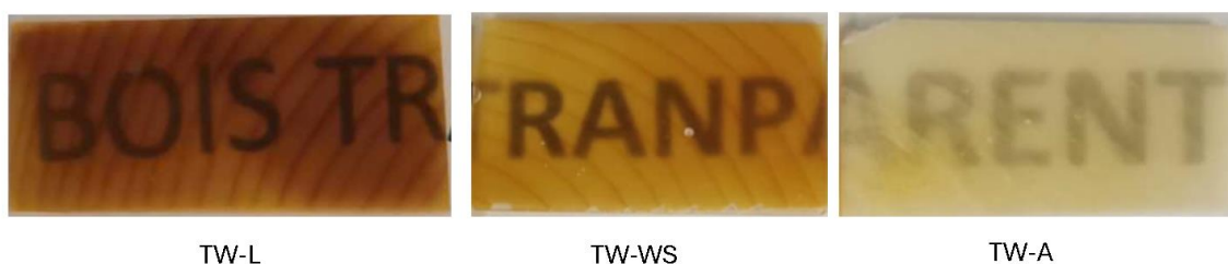
Figure 5. Visual representation of transparent wood from Larch (TW-L), White Spruce (TW-WS), and Aspen (TW-A) showing the wood is darker for higher-density species.
